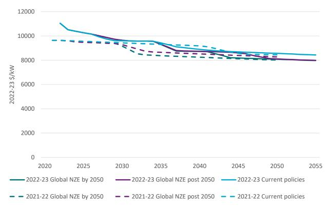
Figure 4-4 Projected capital costs for black coal with CCS by scenario compared to 2021-22 projections
