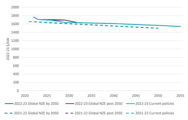
Figure 4-5 Projected capital costs for gas combined cycle by scenario compared to 2021-22 projections
