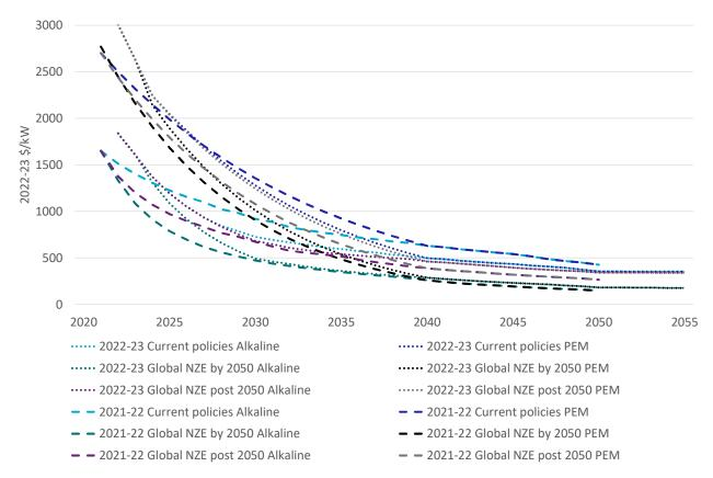
Figure 4-19 Projected technology capital costs for alkaline and PEM electrolysers by scenario, compared to 2021-22
