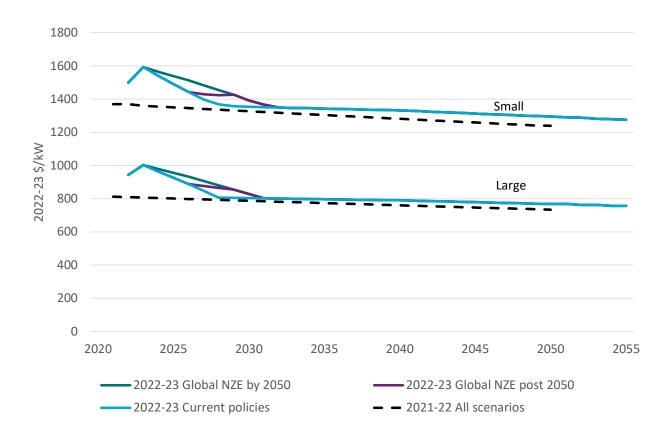
Figure 4-7 Projected capital costs for gas open cycle (small) by scenario compared to 2021-22 projections
