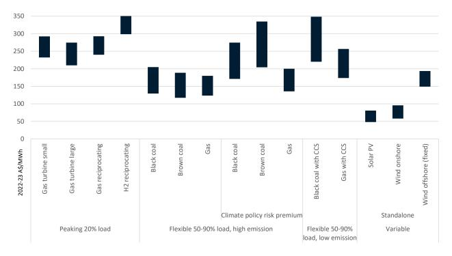
Figure 5-3 Calculated LCOE by technology and category for 2022
