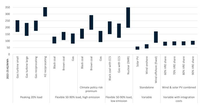
Figure 5-4 Calculated LCOE by technology and category for 2030
