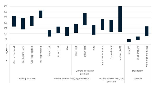
Figure 5-5 Calculated LCOE by technology and category for 2040
