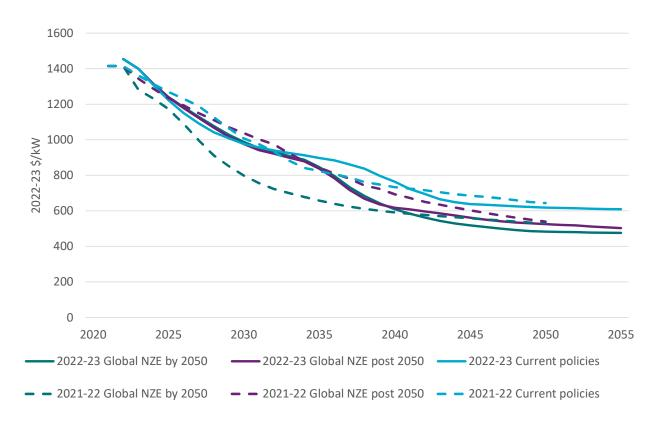
Figure 4-11 Projected capital costs for rooftop solar PV by scenario compared to 2021-22 projections
