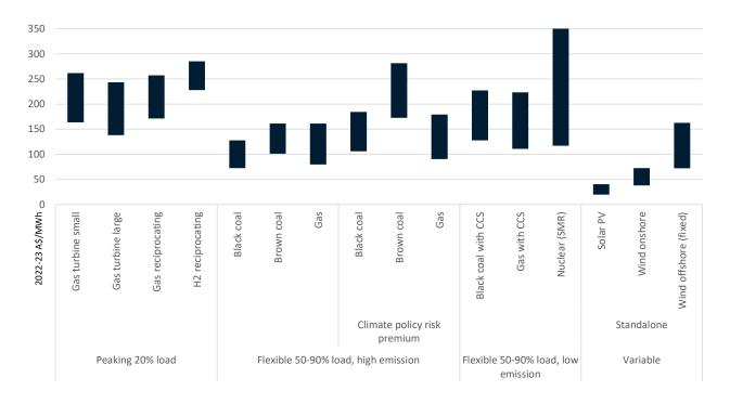
Figure 5-6 Calculated LCOE by technology and category for 2050
