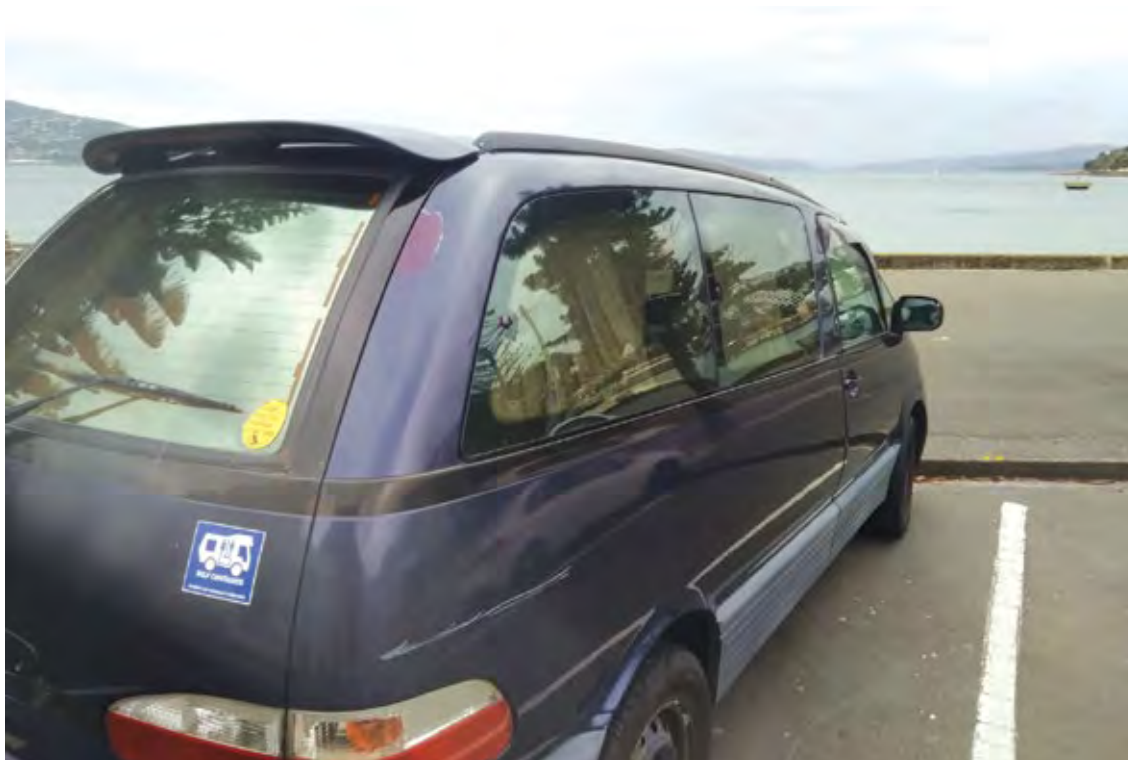
Figure 5.2: The external self-containment sticker used to help identify vehicles that are certified as self-contained under NZS 5465:2001.
